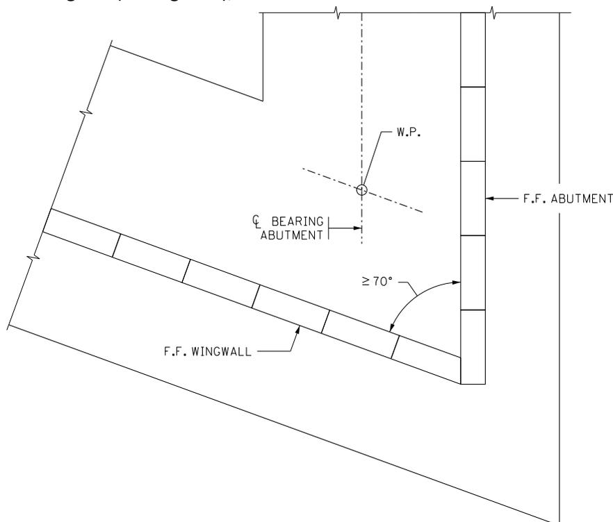
Figure 2: Abutment to Wingwall Angle
