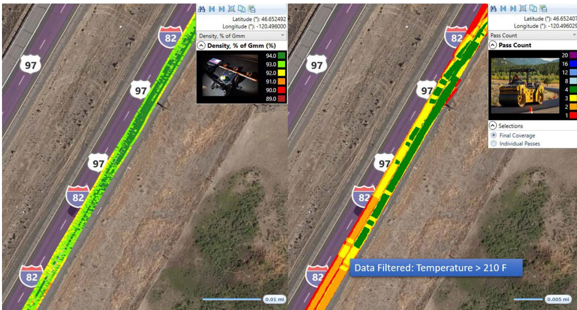
FIGURE 52 Density (left) vs. filtered total pass count (right).
