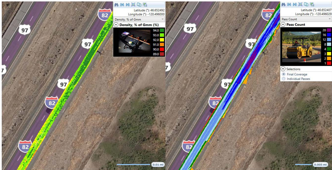
FIGURE 50 Density (left) vs. total pass count (right).
