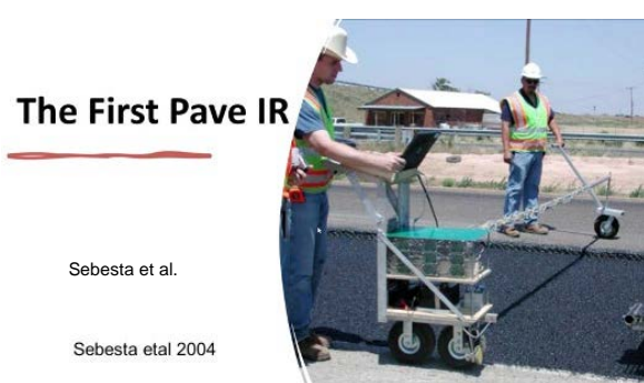
FIGURE 3 First Pave IR system.
