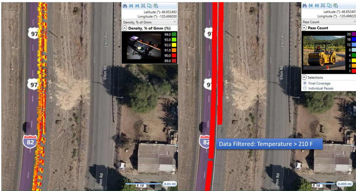
FIGURE 51 Density (left) vs. filtered total pass count (right).
