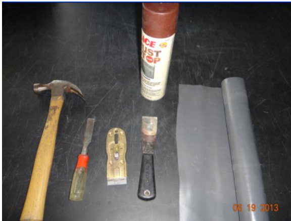
Figure 2.2.1: Vinyl paint sampling tools (spray paint, hammer, chisel, razor scraper, putty knife, and paint collection mat)
