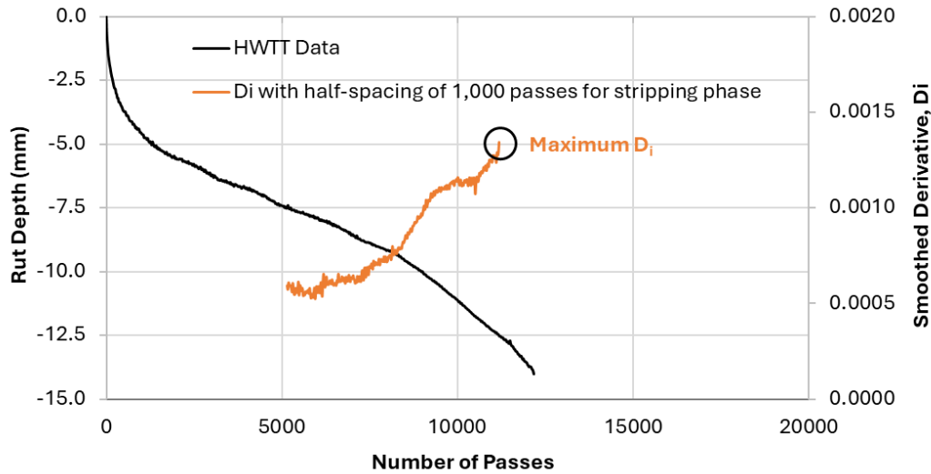
Figure 13. Determining Smoothed Derivative D_i for Method C: (a) using a Half-spacing of 2,000 Passes for Creep Phase, (b) using a Half-spacing of 1,000 Passes for Stripping Phase
