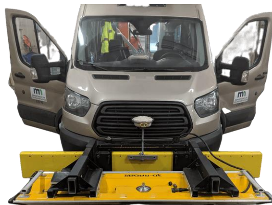
Figure 2. 3D-GPR antenna layout
