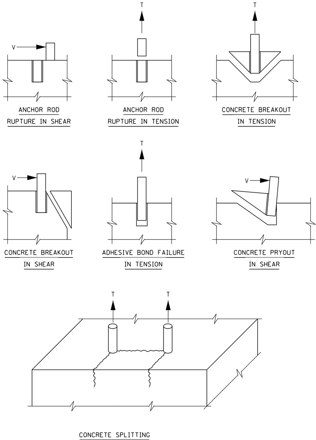
**Adhesive Anchor Failure Modes**
