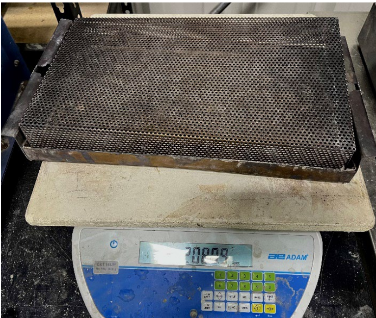
Figure 1. The empty pan and lid placed on a scale covered with heat resistant plate
