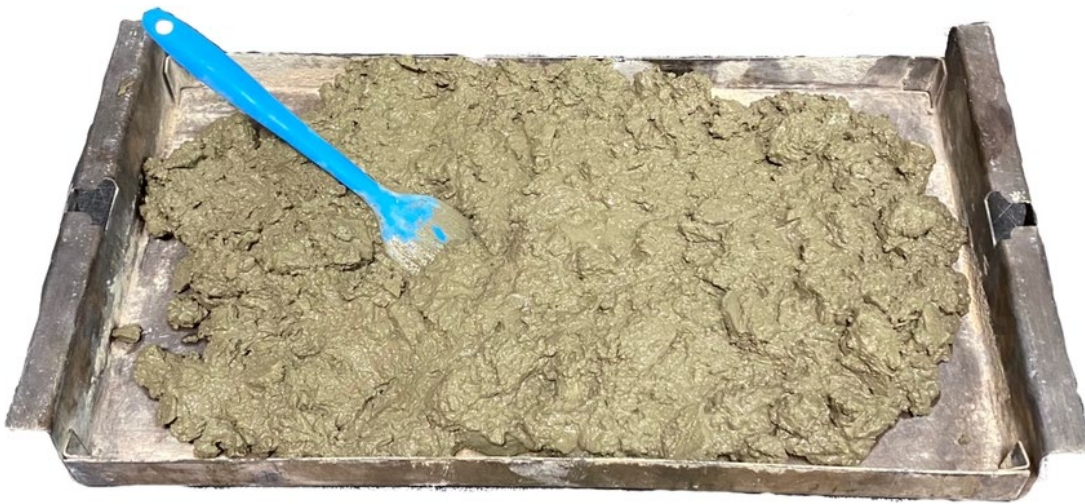
Figure 4. Using a spatula to spread the sample inside the pan
