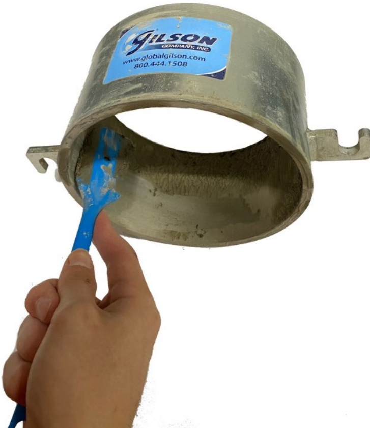
Figure 3. Scraping the cylinder with a spatula
