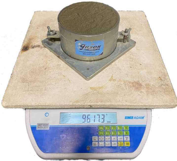
Figure 1. Filled container on a scale covered with a heat resistant plate
