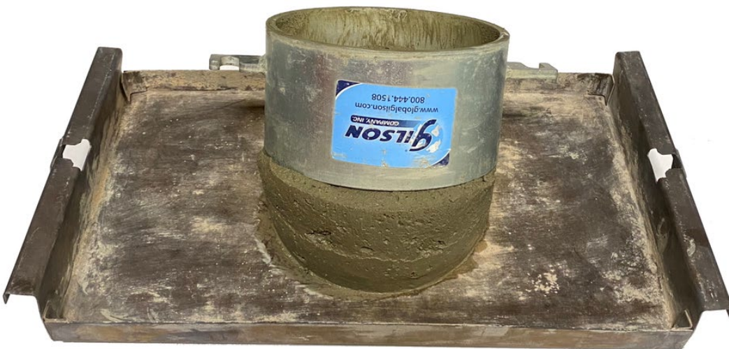
Figure 2. Emptying the cylinder sample into the plate
