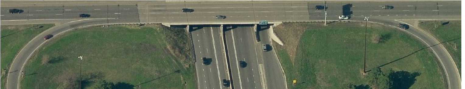
Figure 3: This figure highlights where there is no auxiliary buffer lane (I-494 and I-35W)
