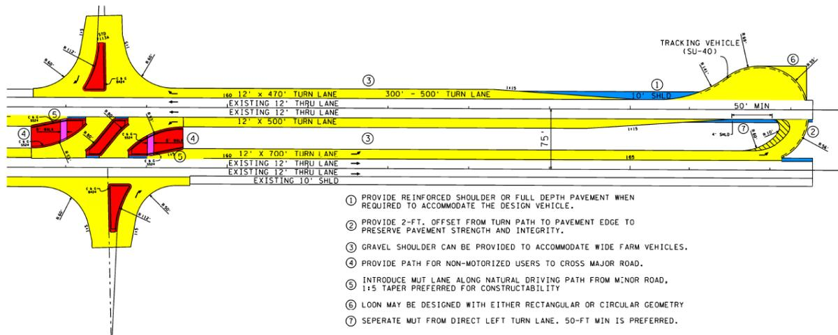
Figure 9 - Typical RCUT Schematic Layout
