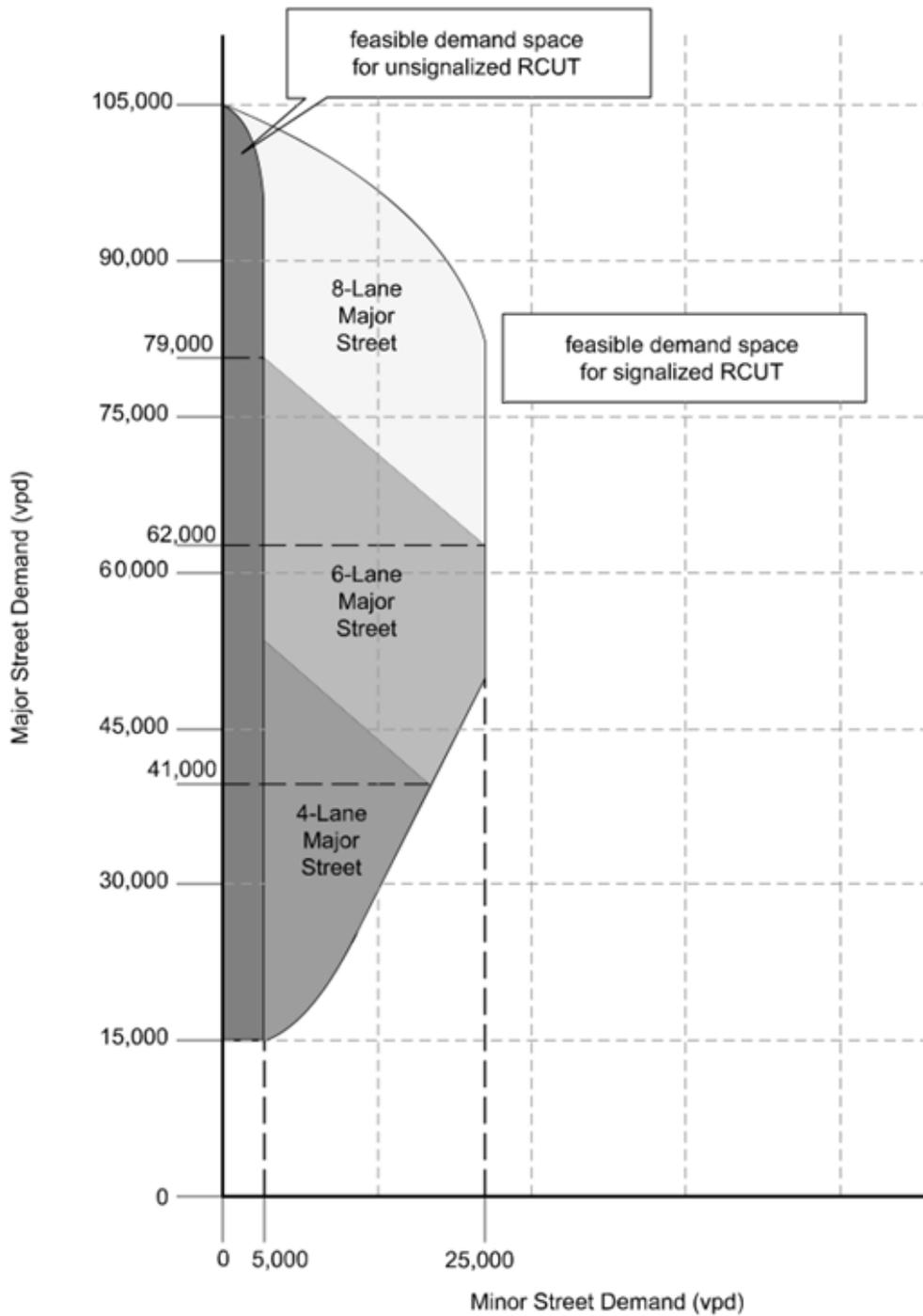
Figure 3 - RCUT Planning Capacity Nomograph
