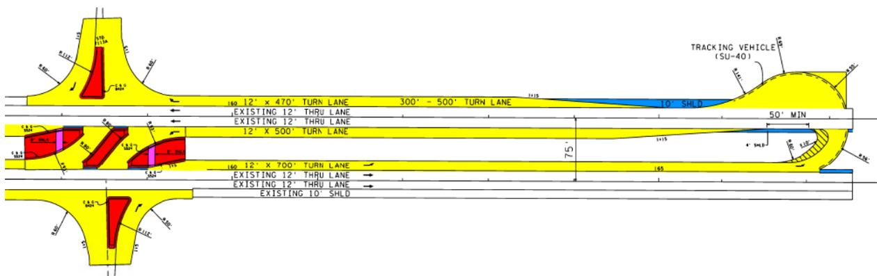
Figure 1: Stop-Controlled RCUT
