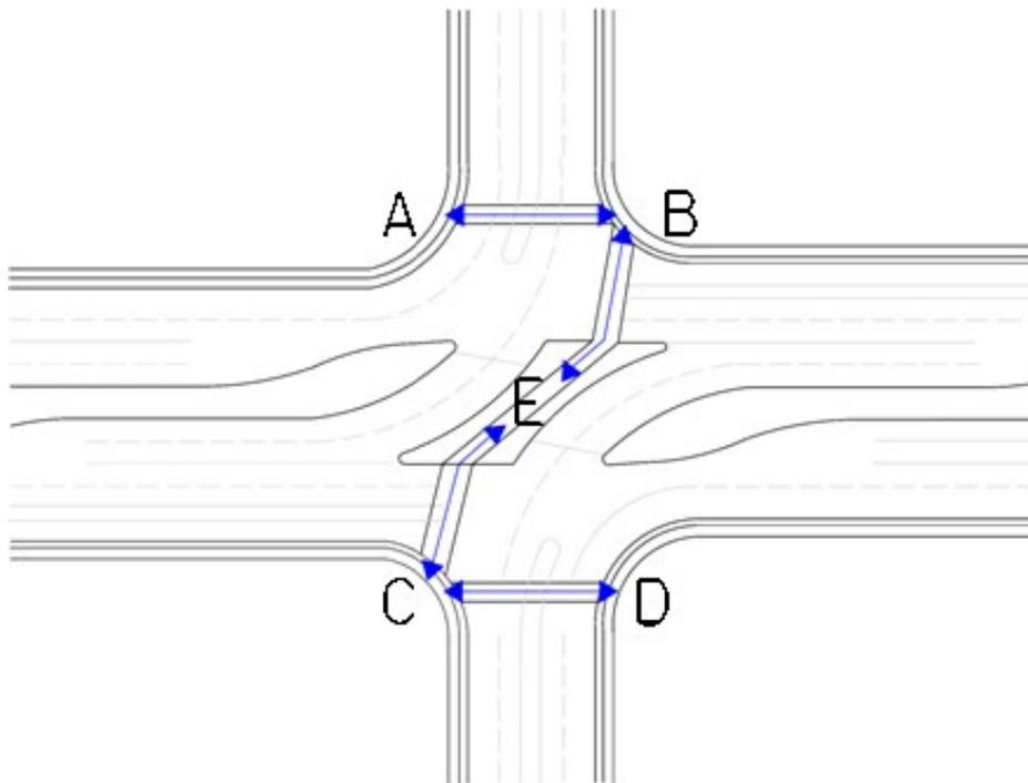
Figure 4 – Z-Crossing Bike and Pedestrian Accommodation in RCUT Intersection (Curb Cut Provided in Raised Median)
