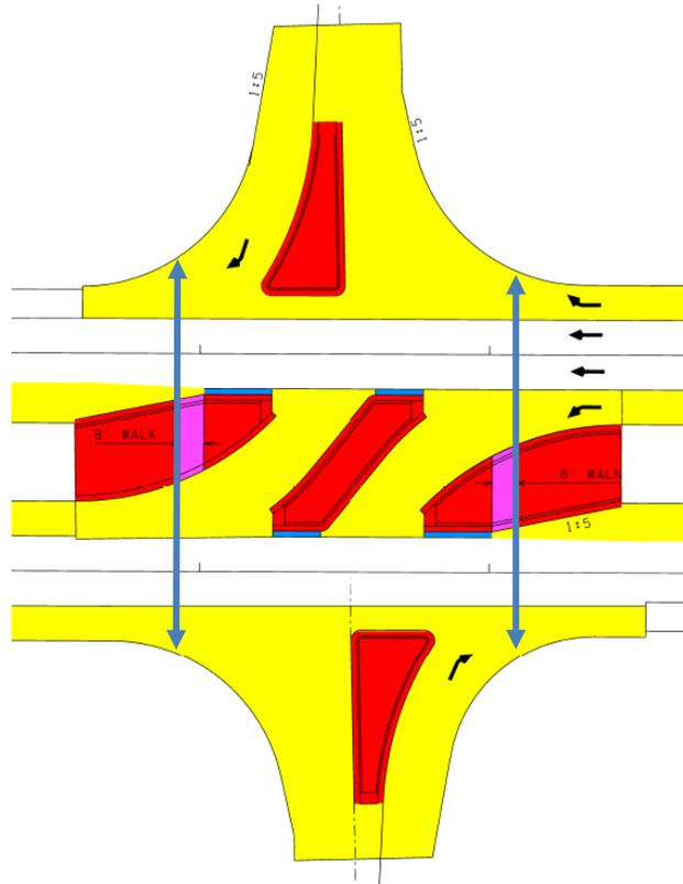
Figure 5 - Direct Pedestrian Crossing in RCUT Intersection
