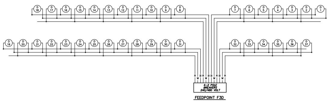
B AND R DENOTE CURRENT CARRYING CONDUCTORS W DENOTES NEUTRAL CONDUCTOR GROUND NOT SHOWN FOR CLARITY
