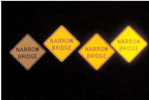
This photo illustrates differences in retroreflectivity between sheeting types.
