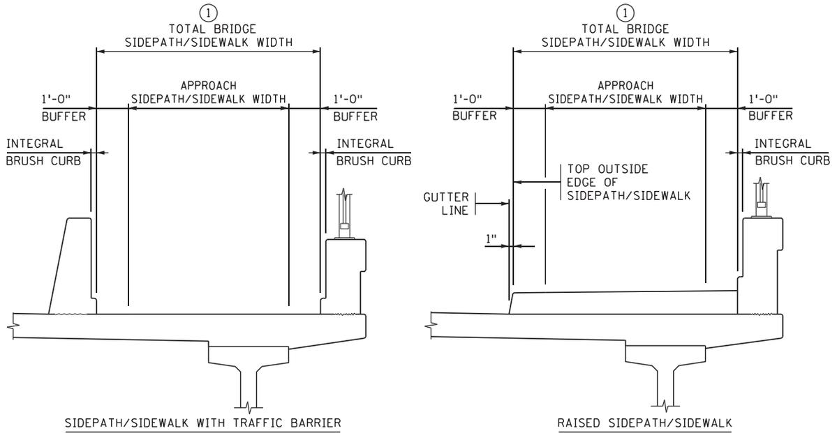
① FOR TOTAL WIDTHS > 10'-0", INTEGRAL BRUSH CURB (MAX. 2" WIDE x 6" HIGH) MAY BE INCLUDED IN TOTAL WIDTH.
