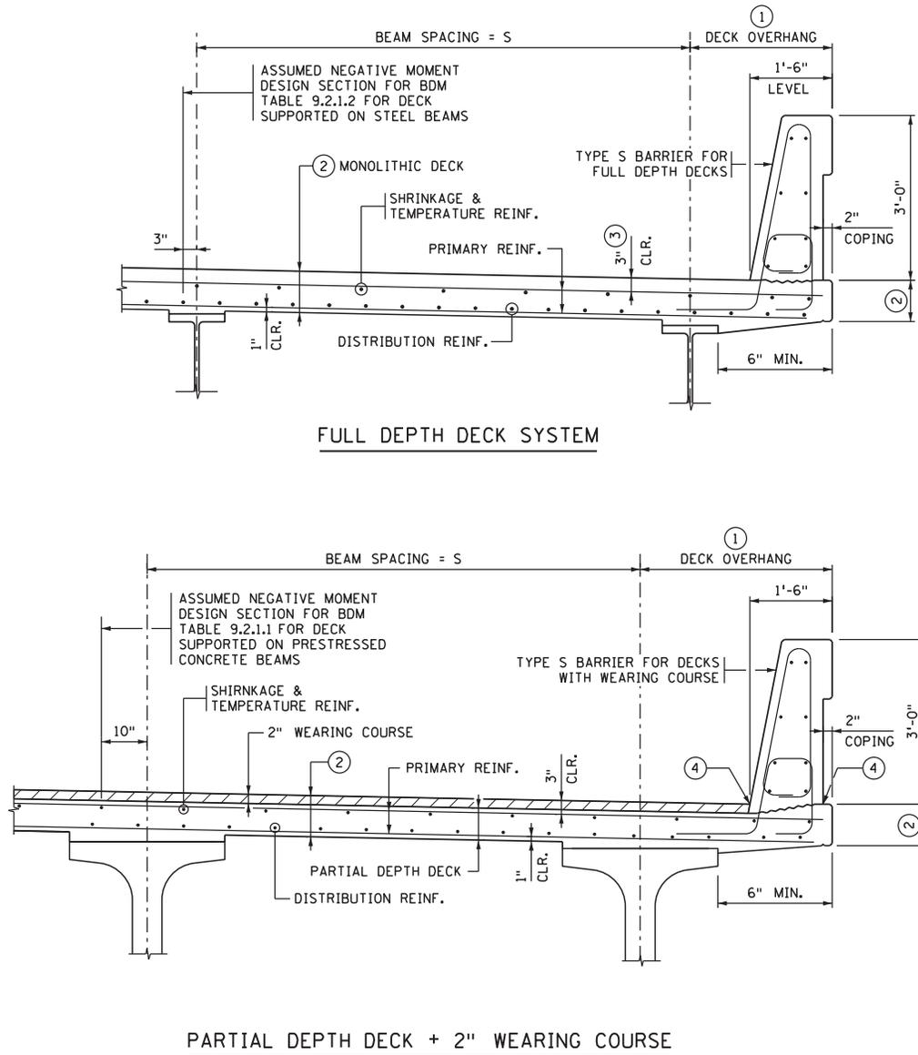
GEOMETRY AND DESIGN ASSUMPTIONS FOR MOST COMMON CONCRETE DECK SYSTEMS
