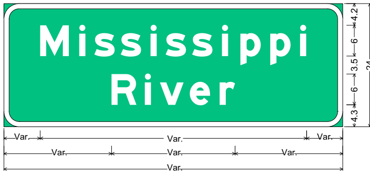
3.0" Radius, 1.0" Border, White on, Green; "Mississippi", E Mod 2K; "River", E Mod 2K;
