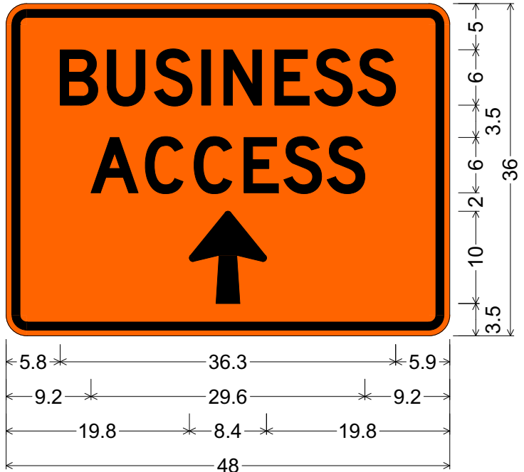
BUSINESS ACCESS UP ARROW; 2.3" Radius, 0.9" Border, 0.6" Indent, Black on Orange; "BUSINESS", D 2K; "ACCESS", D 2K; Arrow 3 - 10.0" 90°;
