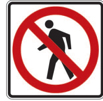
Figure 13-2 No Pedestrian Crossing Sign R9-3 R9-3a
