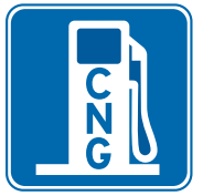
D9-11a Alternative Fuel Compressed Natural Gas
