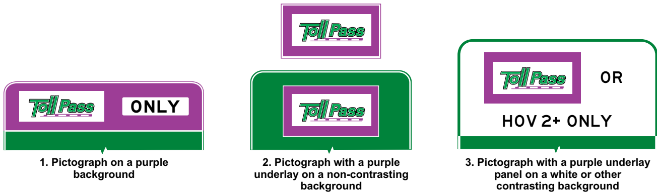
Figure 2F-1 Examples of ETC Account Pictographs and Use of Purple Backgrounds and Underlay Panels
