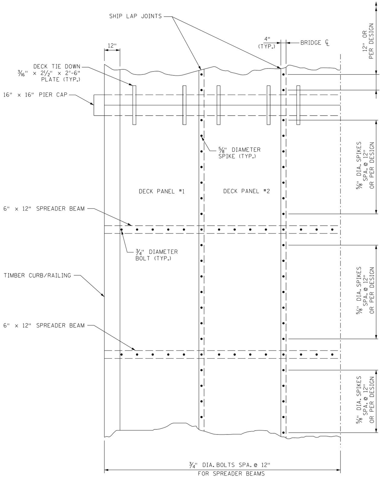
Figure 8.7.1.3 – Longitudinal Timber Deck Partial Plan View
