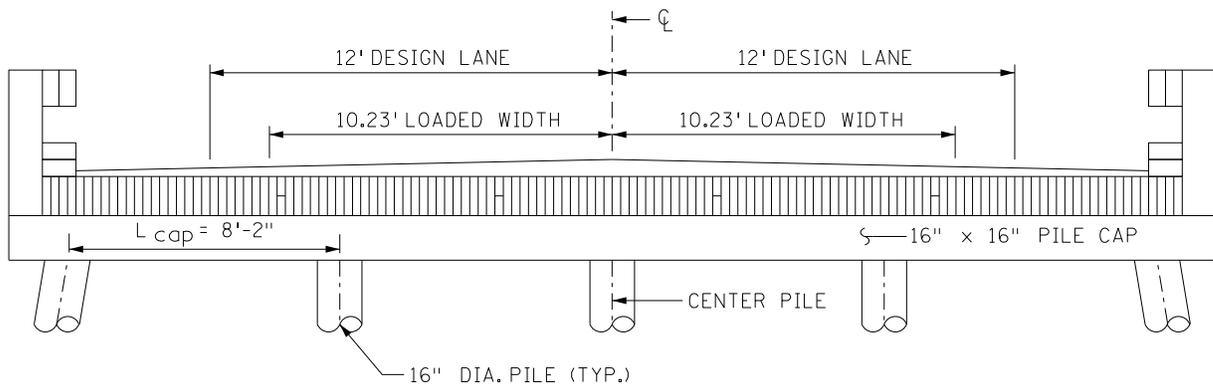
**Figure 8.7.2.2 – Live Load Position for Cap Analysis**
