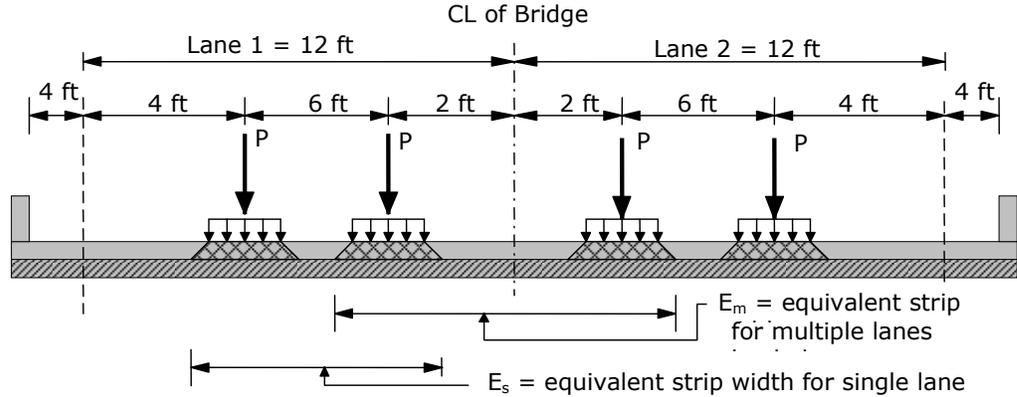
Physical edge-to-edge bridge deck width =  $W = b_{bridge} = 34.0 \text{ ft}$
