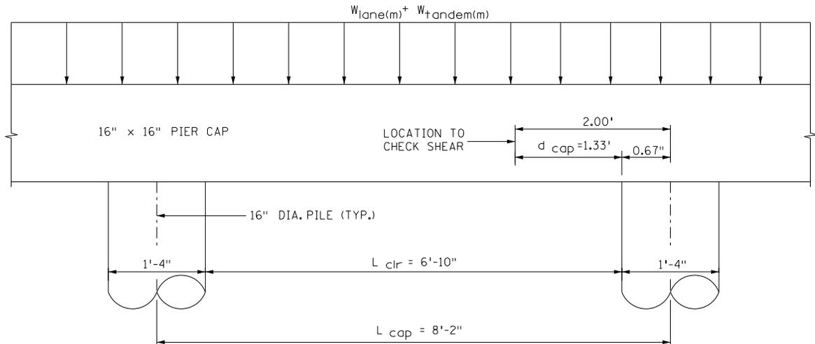
**Figure 8.7.2.3 – Cap Shear Check Location**
