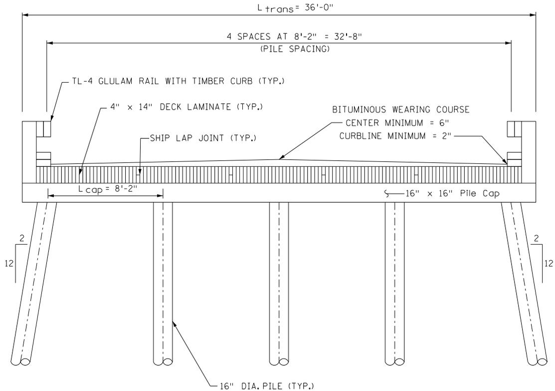
**Figure 8.7.2.1 – Longitudinal Timber Deck on Pier Timber Cap**
