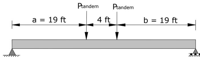
Maximum bending moment due to design tandem axle loads =  $M_{tandem}$
