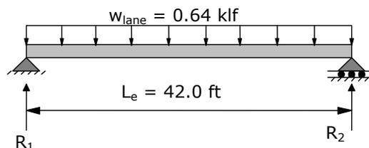
Maximum bending moment due to design lane load =  $M_{\text{lane}}$
