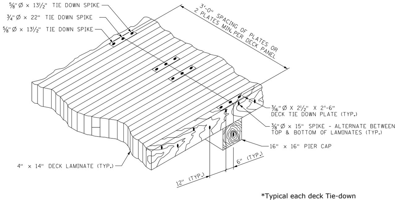
**Figure 8.7.1.2 – Longitudinal Timber Deck to Cap Connections**
