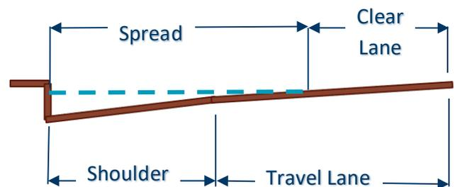
Figure 1: Spread, Clear Lane, Shoulder and Travel Lane Description for use with Table 1.
