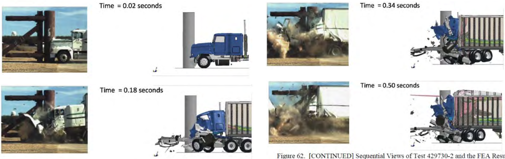
Figure 62. [CONTINUED] Sequential Views of Test 429730-2 and the FEA Results
