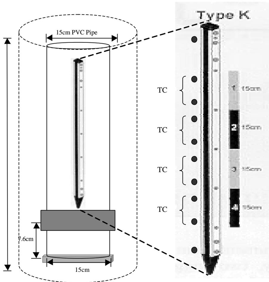
**Figure. 4** Pictured is the Type K Moisture Point probe. The Moisture Point probe is a multi-segment TDR probe with four segments each 15 cm in length. TC = Thermocouple locations in reference to the TDR segments.
