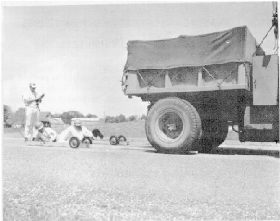
Figure 2. M.H.D. Benkelman Beam
