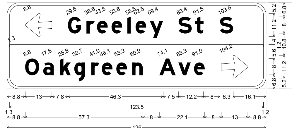
D-43; 6.0" Radius, 1.3" Border, White on Green; Arrow 5 - 13.0" 180°; [Greeley St S] E Mod; [Oakgreen Ave] E Mod; Arrow 5 - 13.0" 0°;
